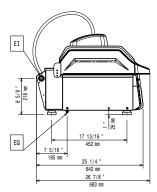
Electrical inlet (power) Electrical Outlet
